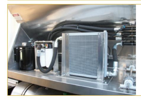
A steel Cyclone hydraulic reservoir packaged on a Midwest General Repair live-bottom trailer. The 20 gpm unit is designed to be significantly smaller than a standard reservoir, which can be a benefit in space-constricted applications, Price Engineering said.
