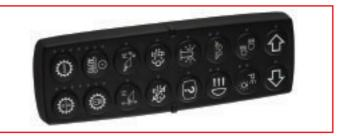
The CL 613/614 keypads have rubber membrane pushbuttons and utilize metal actuation domes for long life exceeding 2 million actuations, HED said. They are offered in two standard form factors — two rows of four buttons or two rows of eight and are available with a variety of LED colors for each button or indicator. The LEDs are dimmable, both as indicators and icon backlights, HED said, and icons are laser-etched and customizable or available off-the-shelf as circular white icons.
